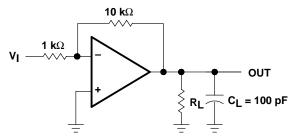
Figure 2. Gain-of-10 Inverting Amplifier
