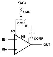
Figure 4. Input Offset Voltage Null Circuit
