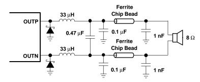
Figure 26. Typical LC Output Filter for 8- $\Omega$  Speaker, Cutoff Frequency of 41 kHz
