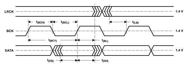
Figure 19. Audio Interface Timing
