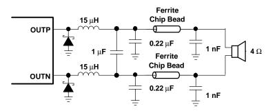
Figure 25. Typical LC Output Filter for 4- $\Omega$  Speaker, Cutoff Frequency of 41 kHz
