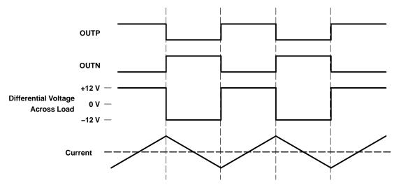
Figure 21. Traditional Class-D Modulation Scheme's Output Voltage and Current Waveforms Into an Inductive Load With No Input
