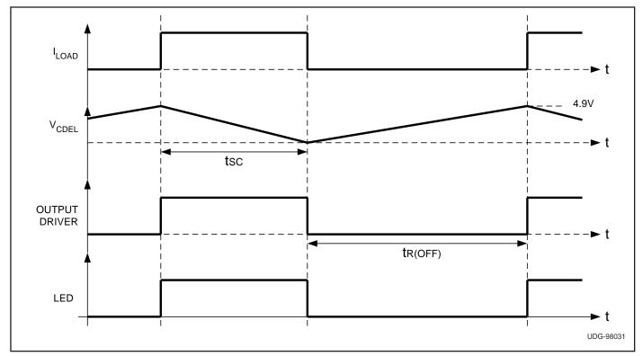
Figure 3c. Overcurrent fault operation.
