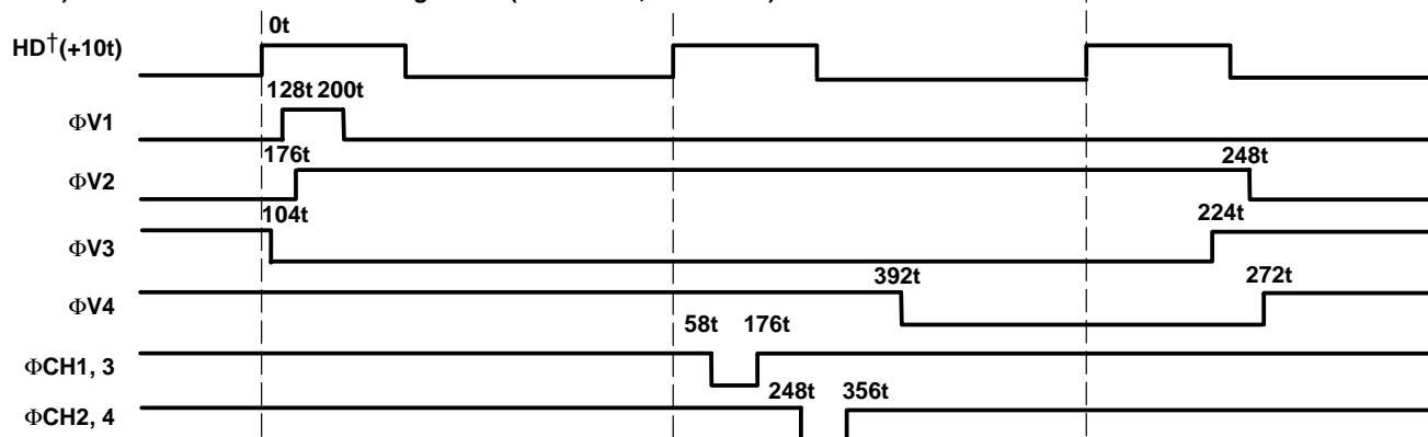
2) V-Rate Readout Detailed Timing Chart: (Field Mode, Even Field)
