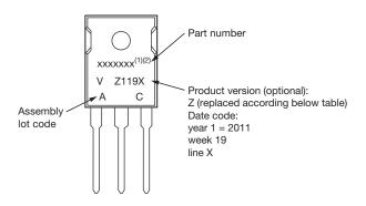
Example: This is a xxxxxxx (1) with assembly lot code AC, assembled on WW 19, 2011 in the assembly line "X"
