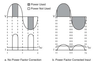
Fig. 1 - Non-PFC vs. PFC Waveforms (Current, Voltage)
