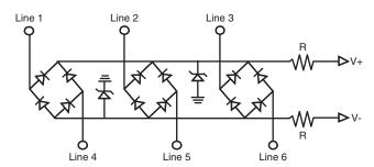
Multiple line protection can be implemented by tying several bridges into one set of TVS's. For single supply systems, one TVS can be eliminated and that node connected to ground.
