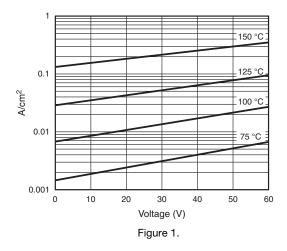
Both the low and high-barrier-height Schottky devices are valuable in a variety of applications. When the true operating temperature of the Schottky rectifier exceeds 125 °C, the high-barrier-height series must be used to avoid thermal runaway.
