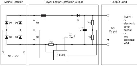
Fig. 4 - Typical Boost Converter Topology for Active PFC
