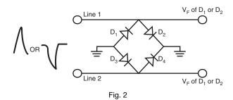
These small components are capable of handling 120 (MBS) and 160 (DFS) A on the industry standard 10 µs/1000 µs current waveform. This is the same waveform that is used to test the axial and surface mount TVS components. For the MB1S the maximum V<sub>F</sub> encountered at 120 A is 7 V hence, it is possible to use the 100 V version of either bridge in this application without fear of reliability issues caused by reverse breakdown of the diodes within the bridge during surge events.
