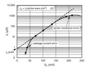
Figure 2. Calculation of J<sub>0</sub> (current density at zero Volts)
