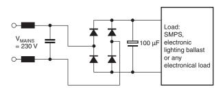
Fig. 1 - Standard Bridge Rectification of Line Voltage
