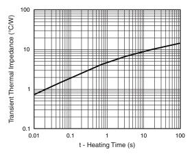
Fig. 6 - Typical Transient Thermal Impedance
