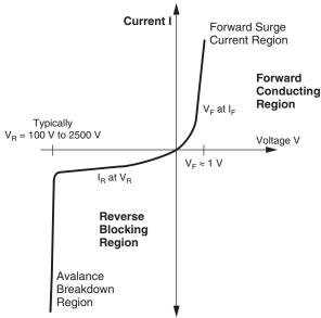
Fig. 1 - Basic Rectifier Characteristics
