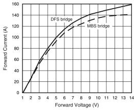
Fig. 1 - Forward Current vs. Forward Voltage
