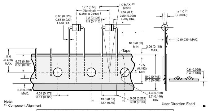
Available only for MPG06 Product in Ammo Pack in Accordance with EIA Standard RS-468-A Utilizing 0.61 mm (0.024") Diameter Leads. Maximum Cumulative Pitch Tolerance: 1.0 mm (0.039")/20 Pitch.
