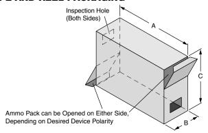
All axial-leaded devices are packed in accordance with EIA standard RS-296-E. The diagrams given below refer to these specifications.
