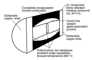
Fig. 1 - SUPERECTIFIER Construction
