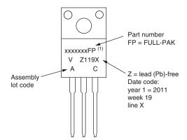
Example: This is a xxxxxxxFP <sup>(1)</sup> with assembly lot code AC, assembled on WW 19, 2011 in the assembly line "X"
