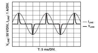
Fig. 2 - 20 W Resistive Load Powered by a Circuit like Fig. 1
