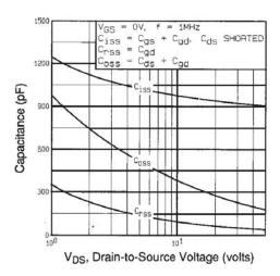
Fig. 5 - Typical Capacitance vs. Drain-to-Source Voltage
