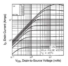
Fig. 1 - Typical Output Characteristics, T<sub>C</sub> = 25 °C
