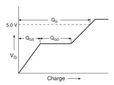
Fig. 13a - Basic Gate Charge Waveform
