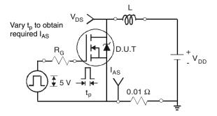
Fig. 12a - Unclamped Inductive Test Circuit
