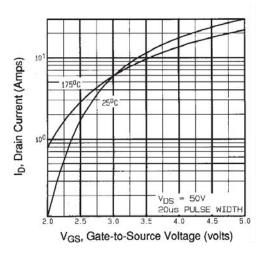
Fig. 3 - Typical Transfer Characteristics
