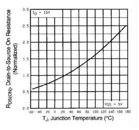
Fig. 4 - Normalized On-Resistance vs. Temperature
