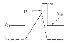
Fig. 12b - Unclamped Inductive Waveforms
