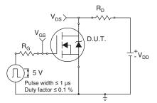
Fig. 10a - Switching Time Test Circuit
