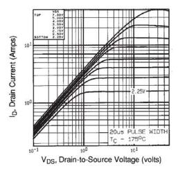
Fig. 2 - Typical Output Characteristics,  $T_C = 175$  °C
