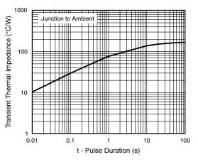
Fig. 6 - Typical Transient Thermal Impedance
