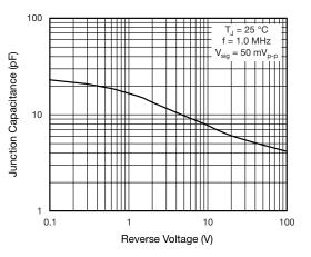
Fig. 5 - Typical Junction Capacitance
