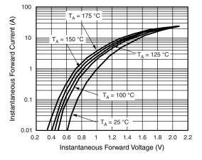
Fig. 3 - Typical Instantaneous Forward Characteristics
