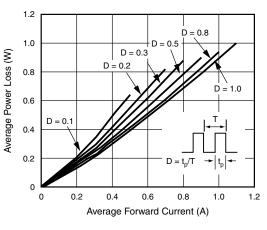
Fig. 2 - Forward Power Loss Characteristics
