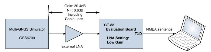
Figure 3-1. Measurement Platform
