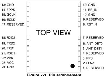
Figure 7-1. Pin arrangement
