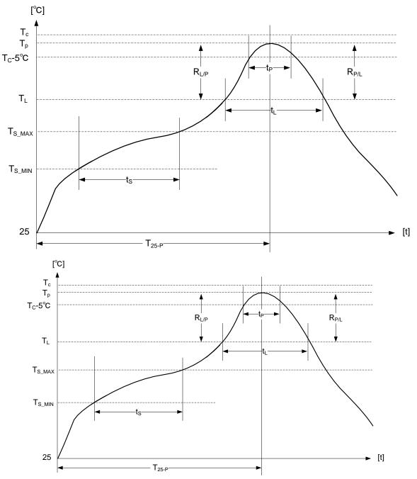
Figure 16-1. Reflow condition
