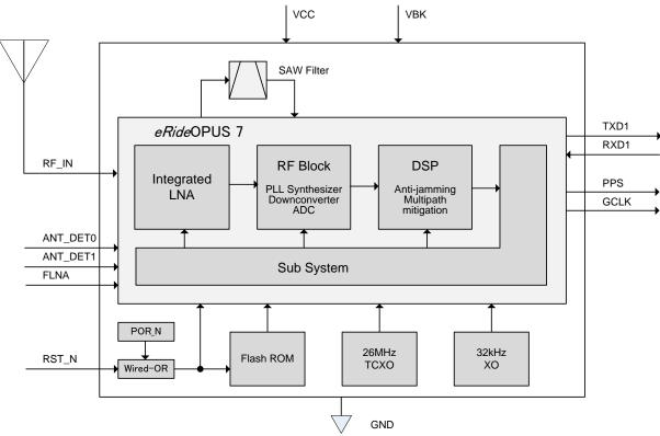
Figure 2-1. Block Diagram
