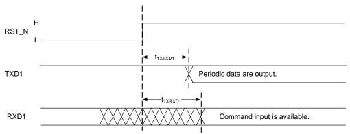
Figure 9.6-2. UART Wake-up Timing after RST\_N
