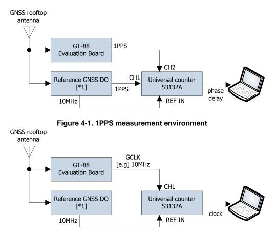
Figure 4-2. GCLK measurement environment
