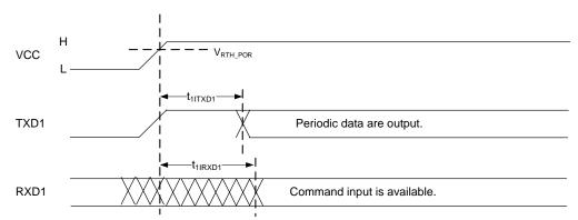
Figure 9.6-1. UART Wake-up Timing after VRTH\_POR
