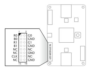
The connector provides a bank of seven I/O pins, which are mapped to the ports as described in the table below:
