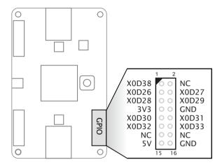
The expansion header provides a bank of nine I/O pins, which are mapped to the ports as described in the table below:
