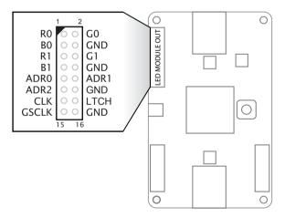
The connector provides a bank of 12 I/O pins, which are mapped to the ports as described in the table on the next page:
