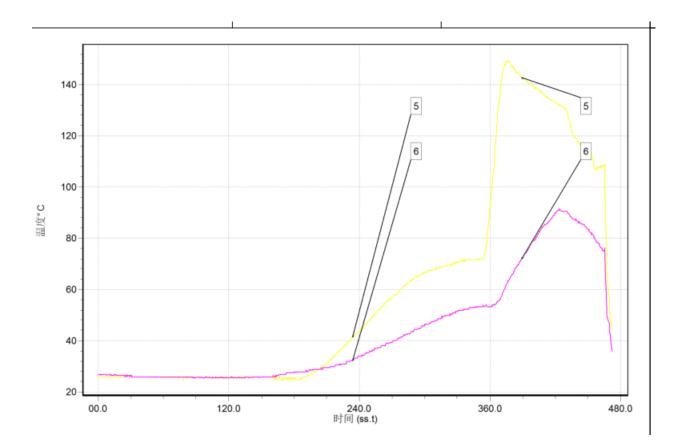
The yellow line (5) shows the temp/seconds for the bottom board, the purple line (6) for above of board.
