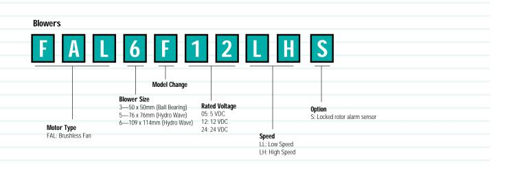
S: Locked rotor alarm sensor
