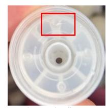
Figure 1. Piston with fine hole defect
