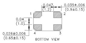
**Note:** Due to the availability of raw materials, this part may be manufactured with the chamfer on pin 4. Be advised that this does not affect the electrical characteristics of the crystal in any way.
