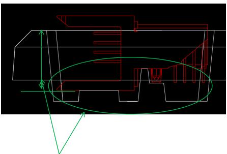
Cavity height improvised & Supporting rib position optimized
