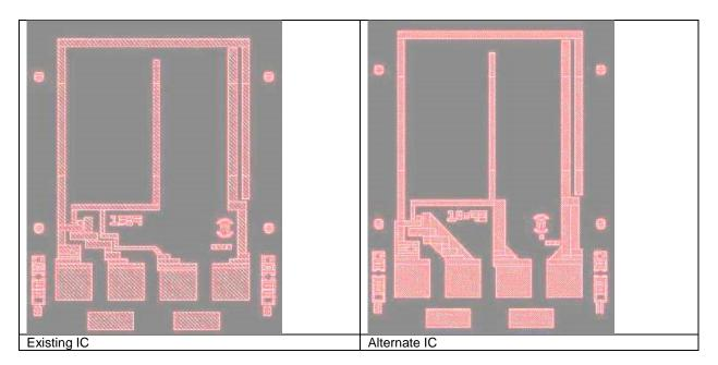
The alternate IC is same as the existing IC, with wider metal trace for improved robustness. No performance change from existing IC.
