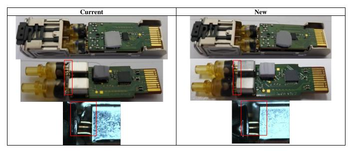
Boxed in red: Current EMI shield has two horns while simplified EMI shield has horns removed.
