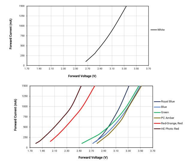
For XQ-E, the current maximum current is 1000 mA. The new maximum current is 1500 mA.
