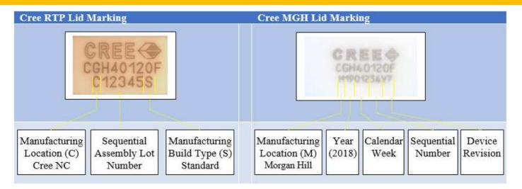
Fabrication of the semiconductor die will not change. GaN-on-SiC die will continue to be fabricated on the Cree campus in North Carolina. The affected RF components are listed below.
