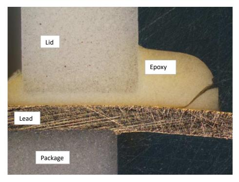
Figure 1. Cross section of a GaN HEMT using prior epoxy.
