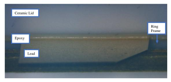
$Figure \ 3. \ Side \ view \ of \ a \ GaN \ HEMT \ using \ the \ new \ epoxy, showing \ a \ tan/butters cotch \ colored \ lid \ seal \ epoxy.$
