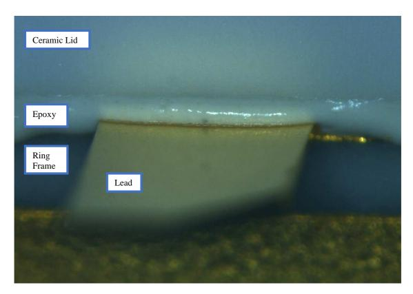
Figure 2. Side view of a GaN HEMT using prior epoxy, showing an off-white colored lid seal epoxy.
