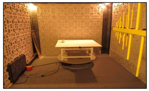
Figure 4 – DUT under Radiated Emissions Test
