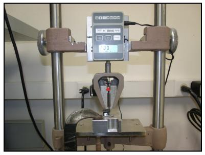
Figure 4– Cable Strength Setup
