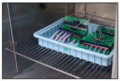
Figure 10 – Operating High Temperature Test Setup
