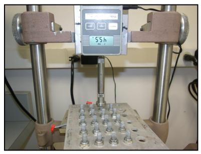
Figure 2– Push Out Force Setup
