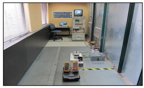
Figure 6 – Conducted Immunity test setup
