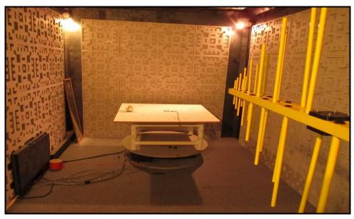
Figure 1 - Radiated Immunity Test Setup
