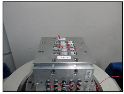
Figure 15 – Random Vibration Test Setup
