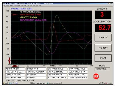
Figure 18 – Mechanical Shock Wave Form
