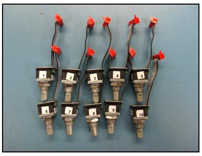
Figure 9 – DUT after Transit Drop
