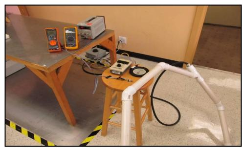
Figure 12 – Magnetic Field Test Setup
