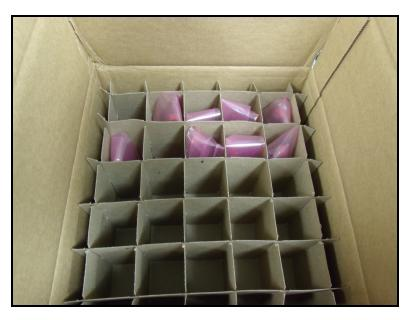
Figure 8 – DUT Packaging after Transit Drop
