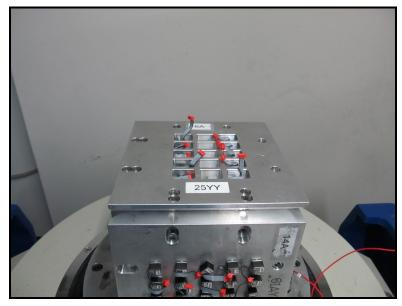
Figure 17 – Mechanical Shock Test Setup
