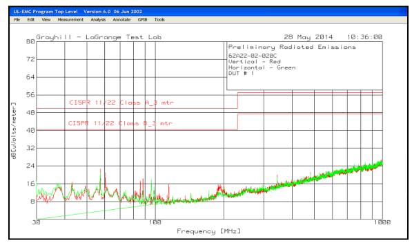
Figure 5 – Radiated Emissions Results (Red Vertical, Green Horizontal)
