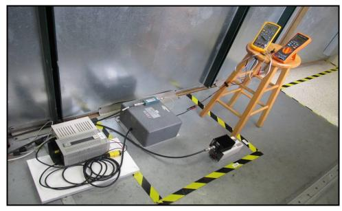
Figure 7 - Conducted Emissions Test Setup
