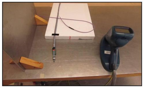
Figure 9 – Electrostatic Discharge Test Setup (Powered)
