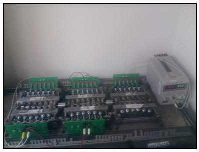
Figure 13 – Push Button Life Test Setup
