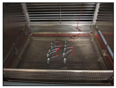
Figure 14 – Thermal Shock Test Setup
