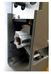
Insert new metal cam in the same orientation as noted in step 4. To start the insertion, make sure the arrow on the cam is pointing toward the center of the unit (toward the solenoid).
