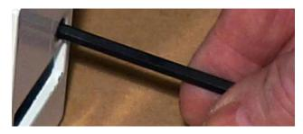
10. Hold up on the locking pin and rotate the new metal cam back and forth a few times to ensure smooth operation and no binding. The operation should feel like what was noted in step 2.
