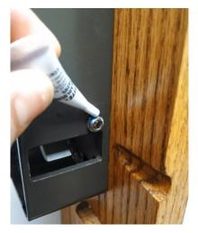
Tighten the two (2) set screws two full revolutions. The face of the set screw should be flush with the side of the interlock housing. If it is not, adjust the set screw to achieve this. Wipe off excess Loctite with a rag.
