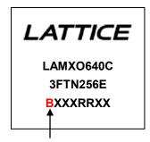
"B" in the first position of Datecode indicates 300mm fab manufactured product
