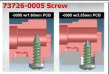
The new screw will have a functional PCB thickness range of 1.6mm to 3.85mm.
