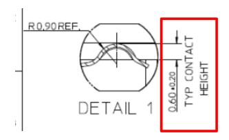
Old Contact Height Specification = 0.60+/-0.20mm New Contact Height Specification = 0.60+0.25/-0.20mm
