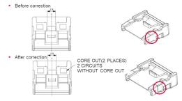
505148 series 2mm pitch FPC to Board connector Plug Jacket Correction of sales drawing
