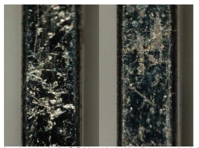
Fig 3. Representative photograph of a C-Grid terminal with reflow matte tin plating after 4000 hours 55 °C / 85% RH exposure per JESD-201 (55X magnification). The terminal on the left is without lead free reflow exposure and terminal on the right was exposed to lead free reflow exposure.
