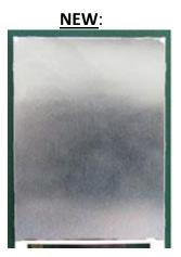
This design change was made to enclose the entire back of the display, covering the exposed backlight reflector which was previously susceptible to damage from external factors.
