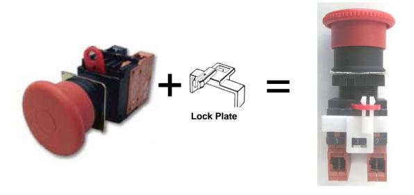
Previously, the A22Z-3380 Lock Plate was available as an accessory to be ordered separately; however, to improve the safety of the switch by protecting it against accidental or unintended removal, the locking plate is now shipped with all A22E\_ Emergency Stop Switches. The change started in Japan in February 2008 and has rolled out worldwide as stock turned over.
