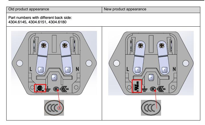
Please note that only screw mounting types are ilustrated. However, the same changes apply to both mounting types with screw flange and snap-in as listed in the affected part numbers list in chapter 1.
