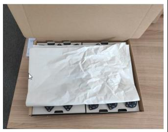
New Box dimension: 365x275x50 mm New Partion 2x25 division: 271x179x37 mm Stuffing paper: 375X500 mm
