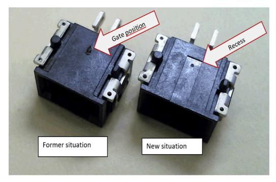
There are actually existing housings from other molds without gate on the bottom side. These housings were not affected.
