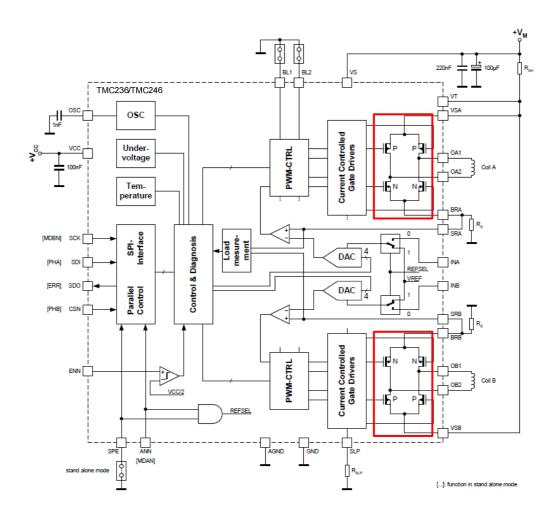
Figure 1: TMC236 block diagram
