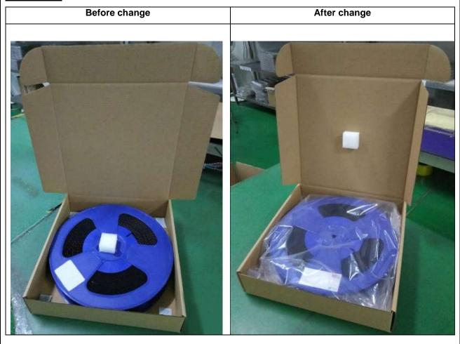
In order to increment oxidation resistance of the packaging in storage, PE bag and desiccant are added to each reel (details on figures above).
