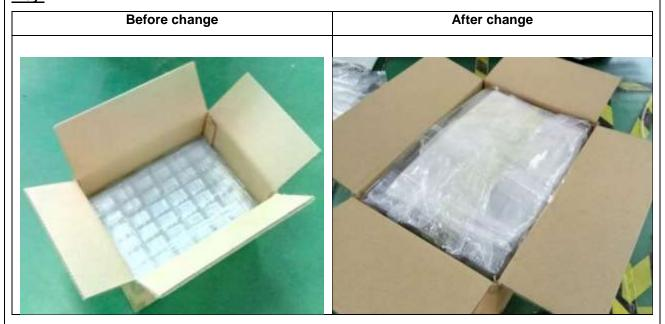
In order to increment oxidation resistance of the packaging in storage, PE bag and desiccant are added to each batch of trays (details on figures above).
