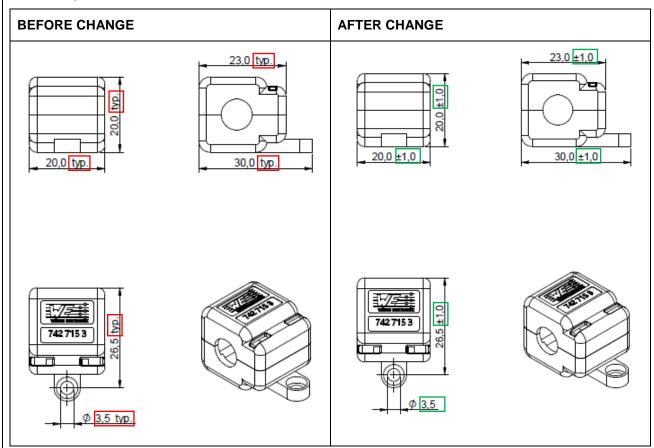
2. Change: General Tolerance Standard from DIN ISO 2768-1m to DIN ISO 2768-1c
