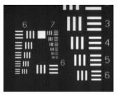
USAF-Testchart exposure with a Dalsa Piranha HS 12k in area-mode and 430 nm illumination. Element 6 of group 7 could be resolved, which means up to 228 lp/mm at a field of view of 17.8 mm.
