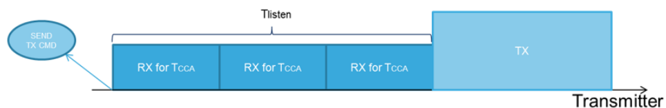
Figure 23. CSMA if channel is free (timeline)
