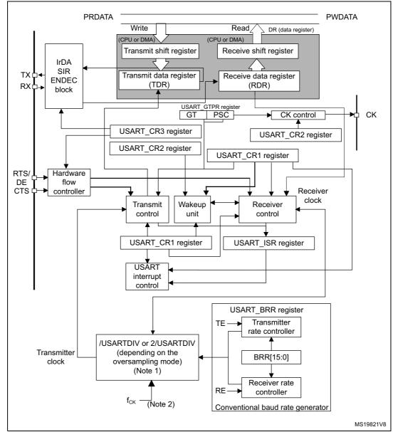
Figure 213. USART block diagram
