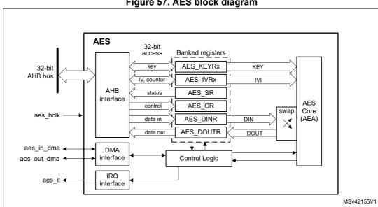
Figure 57. AES block diagram
