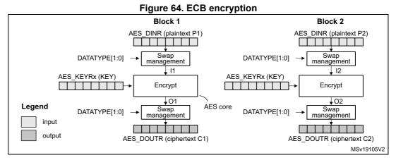
In ECB encrypt mode, the 128-bit plaintext input data block Px in the AES\_DINR register first goes through bit/byte/half-word swapping. The swap result Ix is processed with the AES core set in encrypt mode, using a 128-bit key. The encryption result Ox goes through bit/byte/half-word swapping, then is stored in the AES\_DOUTR register as 128-bit ciphertext
