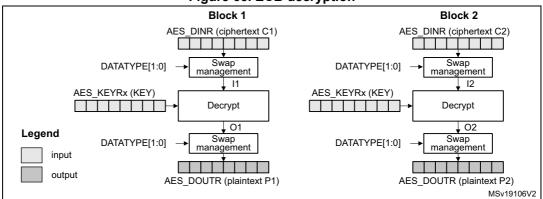
To perform an AES decryption in the ECB mode, the secret key has to be prepared by collecting the last-round encryption key (which requires to first execute the complete key schedule for encryption), and using it as the first-round key for the decryption of the ciphertext. This preparation is supported by the AES core.
