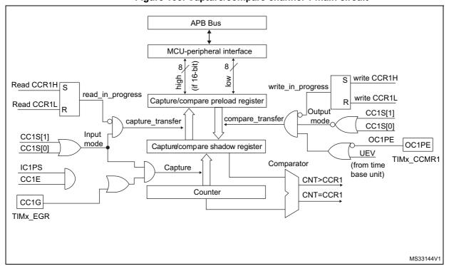
Figure 103. Capture/compare channel 1 main circuit
