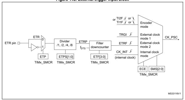
Figure 145. External trigger input block
