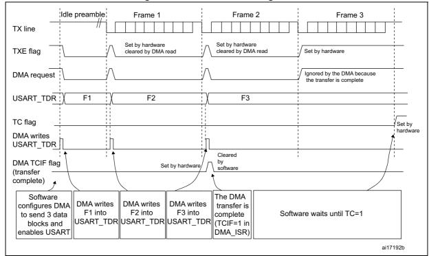
Figure 232. Transmission using DMA
