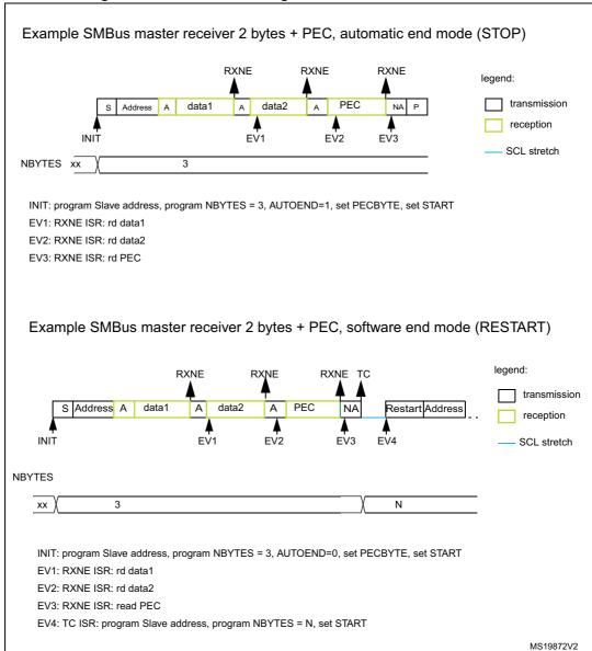
Figure 212. Bus transfer diagrams for SMBus master receiver
