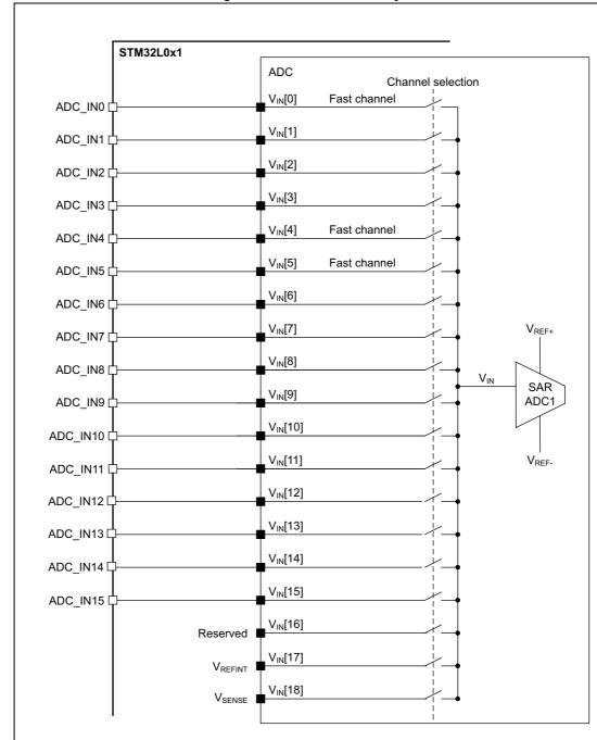
Figure 34. ADC connectivity
