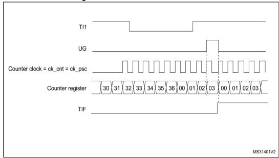
Figure 158. Control circuit in reset mode
