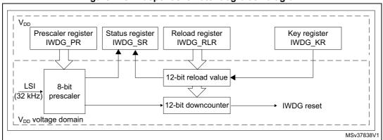
Figure 178. Independent watchdog block diagram
