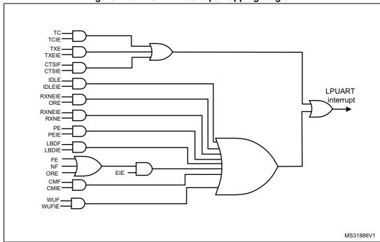
Figure 249. LPUART interrupt mapping diagram
