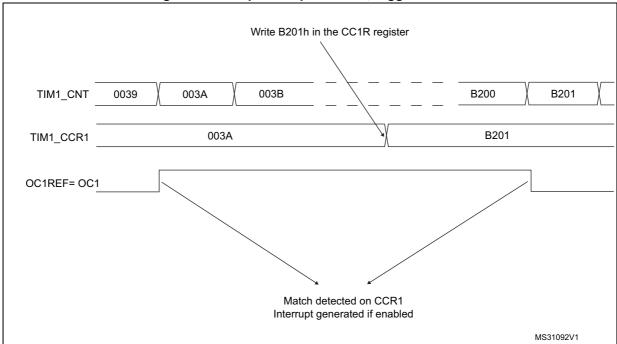
Figure 106. Output compare mode, toggle on OC1.
