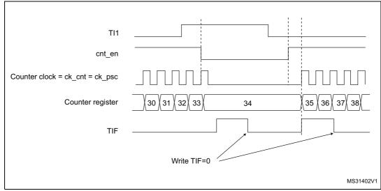
Figure 159. Control circuit in gated mode
