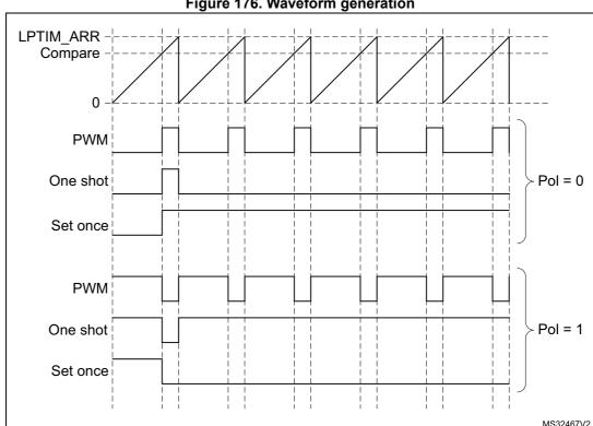
Figure 176. Waveform generation
