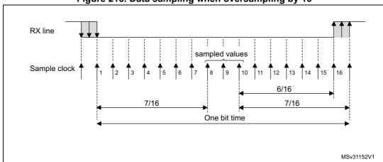
Figure 218. Data sampling when oversampling by 16
