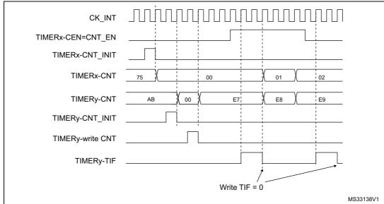
Figure 119. Gating timer y with Enable of timer x
