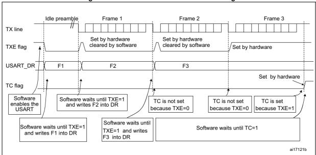
Figure 216. TC/TXE behavior when transmitting
