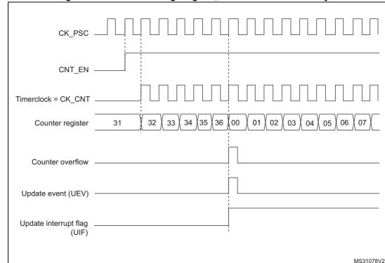
Figure 164. Counter timing diagram, internal clock divided by 1
