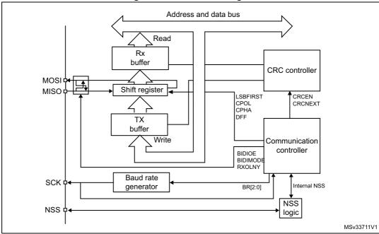
Figure 250. SPI block diagram
