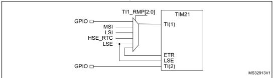
TIM21 has an input multiplexer that selects which of the I/O or the internal clock is to trigger the input capture. This selection is performed through the TI1\_RMP [2:0] bits in the TIM21\_OR register.
