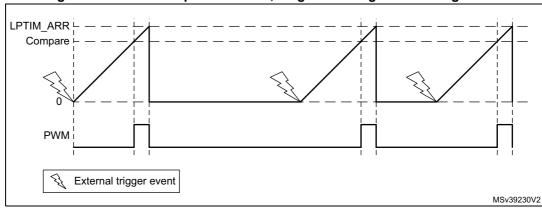
Figure 173. LPTIM output waveform, single counting mode configuration
