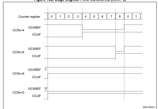
Figure 152. Edge-aligned PWM waveforms (ARR=8)
