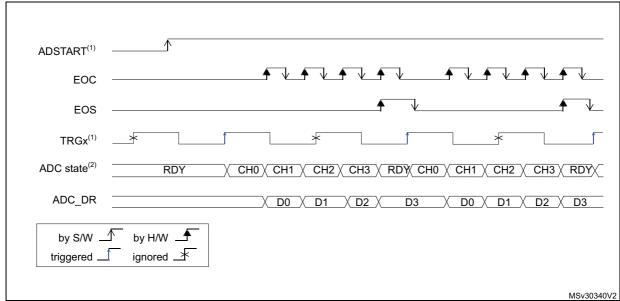
Figure 40. Single conversions of a sequence, hardware trigger
