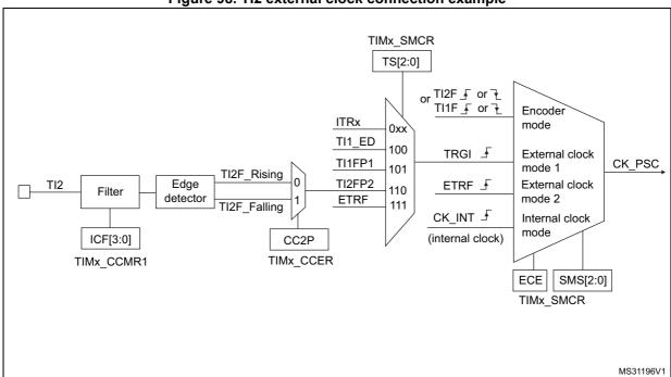
Figure 98. TI2 external clock connection example
