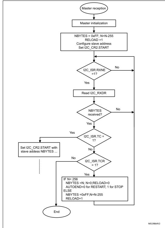
Figure 204. Transfer sequence flow for I2C master receiver for N >255 bytes
