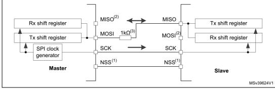
Figure 252. Half-duplex single master/ single slave application
