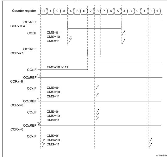
Figure 153. Center-aligned PWM waveforms (ARR=8)
