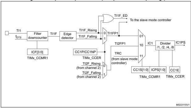
Figure 147. Capture/compare channel (example: channel 1 input stage)
