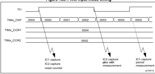
Figure 150. PWM input mode timing
