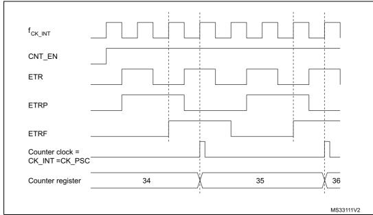
Figure 101. Control circuit in external clock mode 2
