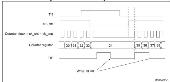
Figure 114. Control circuit in gated mode
