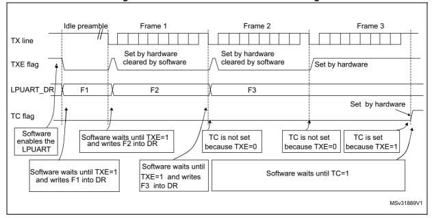
Figure 241. TC/TXE behavior when transmitting
