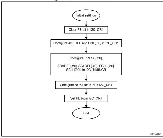
Figure 186. I2C initialization flow
