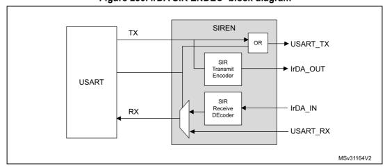
Figure 230. IrDA SIR ENDEC- block diagram
