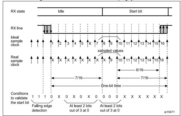
Figure 217. Start bit detection when oversampling by 16 or 8
