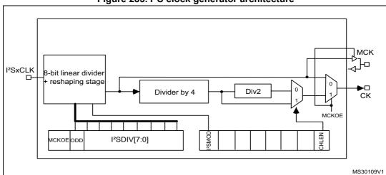
Figure 283. I<sup>2</sup>S clock generator architecture
