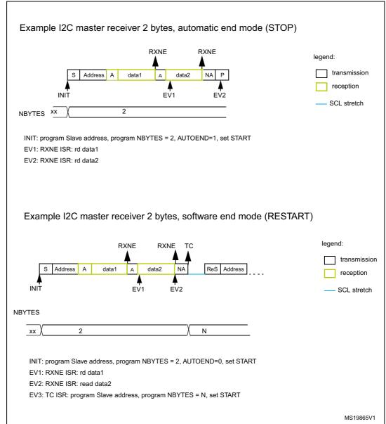
Figure 205. Transfer bus diagrams for I2C master receiver
