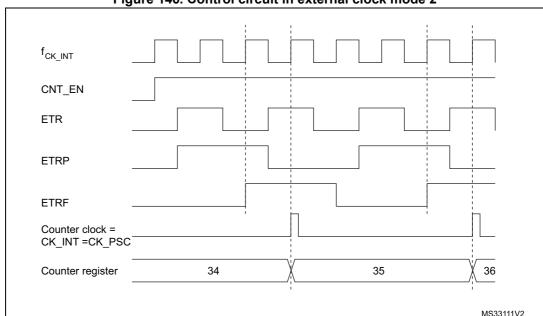
Figure 146. Control circuit in external clock mode 2
