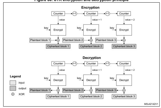
Figure 60. CTR encryption and decryption principle
