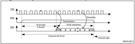
When 16-bit data frame extended to 32-bit channel frame is selected during the I<sup>2</sup>S configuration phase, Only one access to the SPIx\_DR register is required. The 16 remaining bits are forced by hardware to 0x0000 to extend the data to 32-bit format. In this case it corresponds to the half-word MSB.
