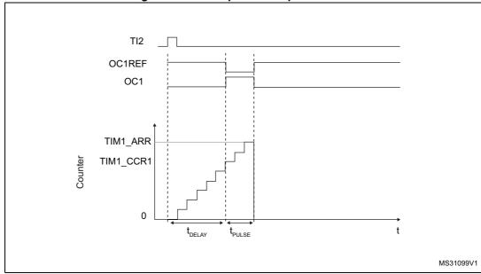
Figure 109. Example of one-pulse mode.
