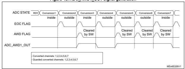
Figure 48. ADC\_AWD1\_OUT signal generation
