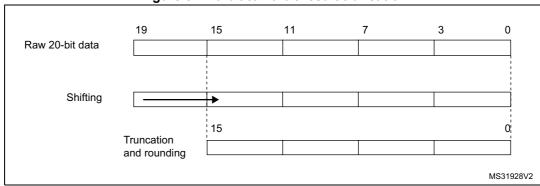
Figure 52. 20-bit to 16-bit result truncation
