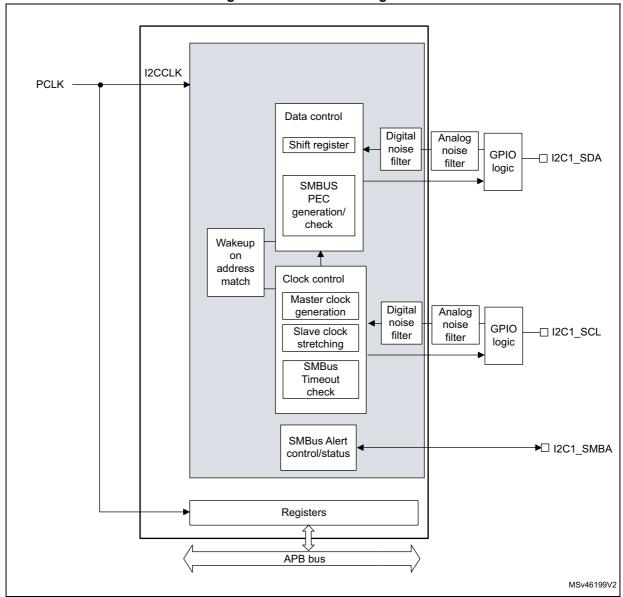
Figure 183. I2C2 block diagram
