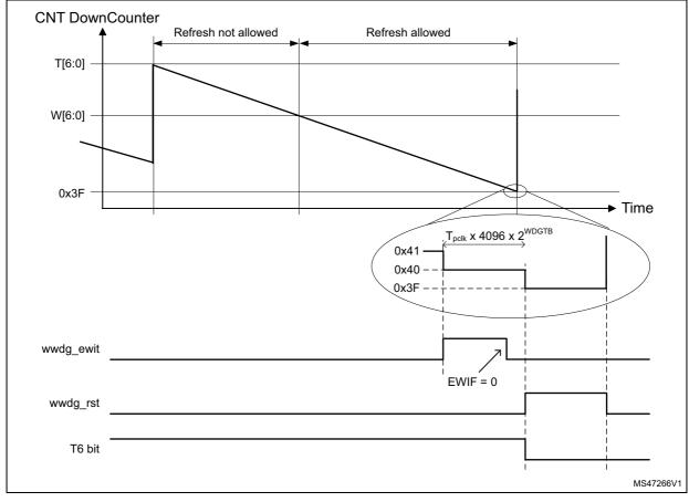
Figure 180. Window watchdog timing diagram
