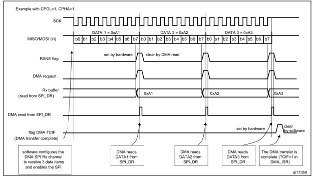
Figure 261. Reception using DMA
