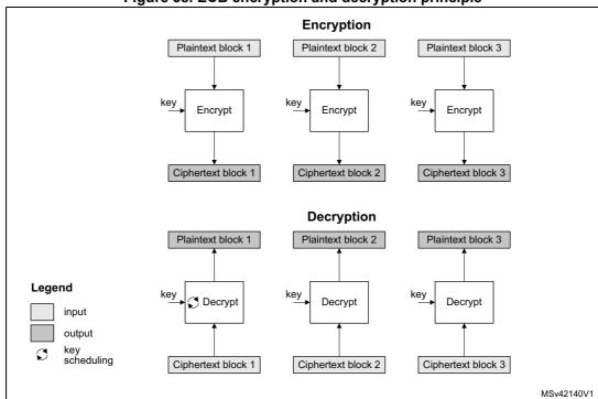
ECB is the simplest mode of operation. There are no chaining operations, and no special initialization stage. The message is divided into blocks and each block is encrypted or decrypted separately.
