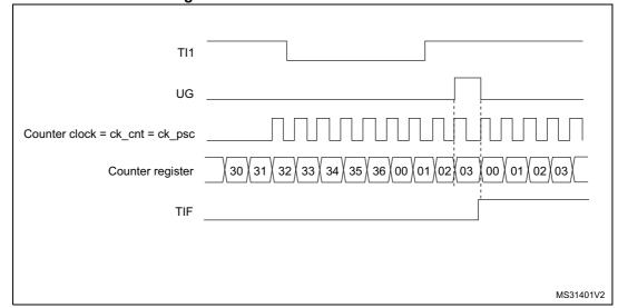
Figure 113. Control circuit in reset mode
