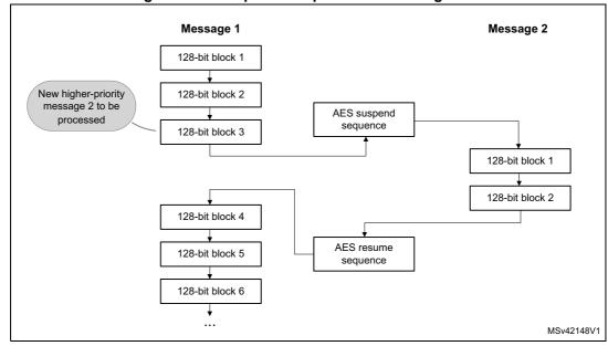
Figure 63. Example of suspend mode management
