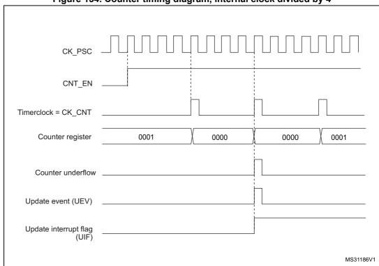
Figure 134. Counter timing diagram, internal clock divided by 4
