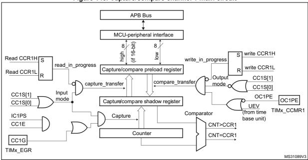
Figure 148. Capture/compare channel 1 main circuit
