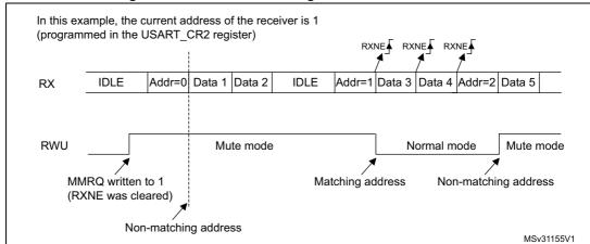
Figure 221. Mute mode using address mark detection
