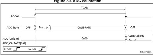
Figure 30. ADC calibration
