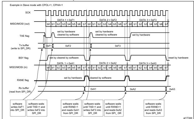
Figure 259. TXE/RXNE/BSY behavior in slave / full-duplex mode (BIDIMODE=0, RXONLY=0) in the case of continuous transfers
