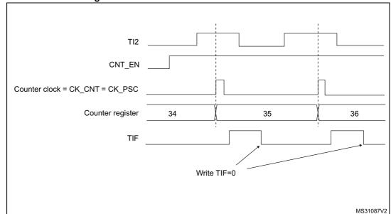
Figure 99. Control circuit in external clock mode 1
