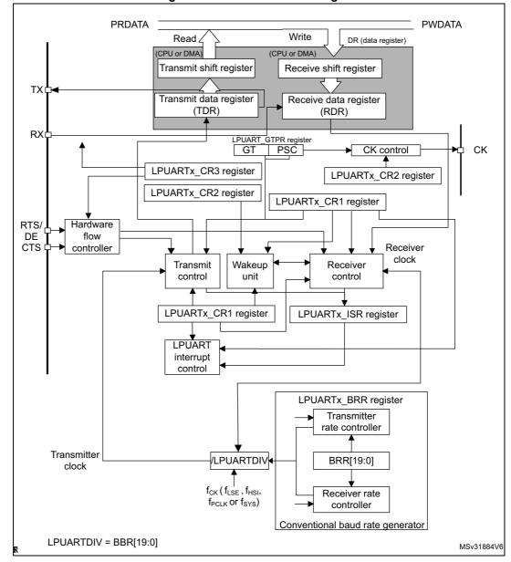
Figure 238. LPUART block diagram
