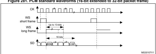
Figure 281. PCM standard waveforms (16-bit extended to 32-bit packet frame)
