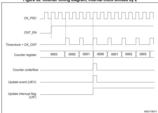
Figure 92. Counter timing diagram, internal clock divided by 2
