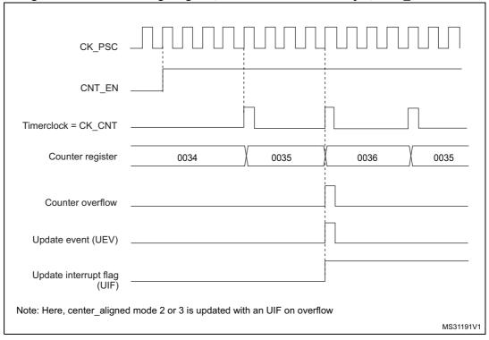
1. Center-aligned mode 2 or 3 is used with an UIF on overflow.
