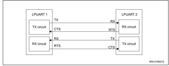
Figure 246. Hardware flow control between 2 LPUARTs
