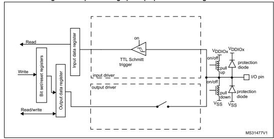
Figure 21. Input floating / pull up / pull down configurations
