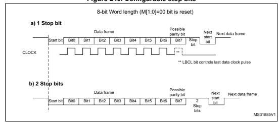
Figure 240. Configurable stop bits
