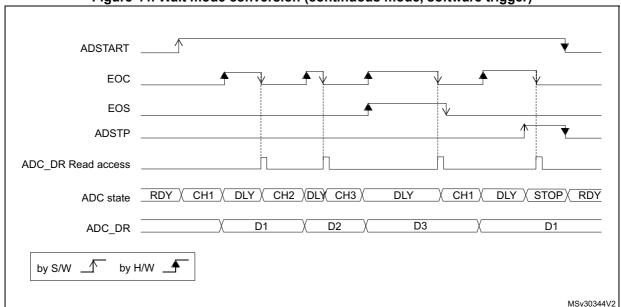
Figure 44. Wait mode conversion (continuous mode, software trigger)
