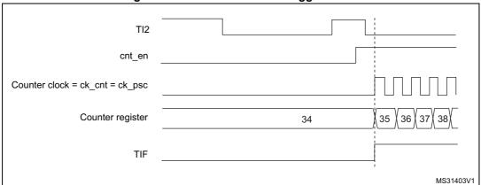
Figure 160. Control circuit in trigger mode
