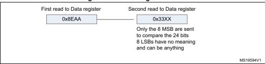
Figure 269. I<sup>2</sup>S Philips standard (16-bit extended to 32-bit packet frame with CPOL = 0)
