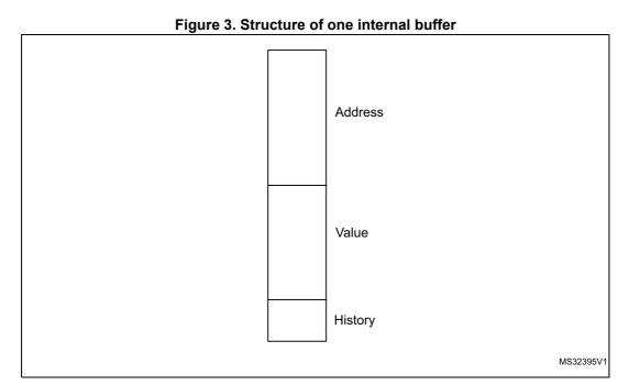
Each buffer stores 3 different types of information: address, data and history. In a read operation, if the address is found, the memory interface can return data without accessing the NVM. Data in the buffer is 32 bit wide (even if the master only reads 8 or 16 bits), so that a value can be returned whatever the size used in a previous reading. The history is used to know if the content of a buffer is valid and to delete (with a new value) the older one.
