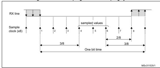
Figure 219. Data sampling when oversampling by 8
