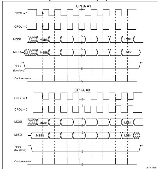
Figure 257. Data clock timing diagram
