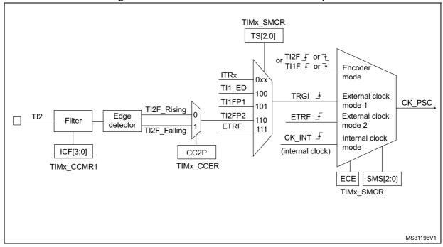
Figure 143. TI2 external clock connection example
