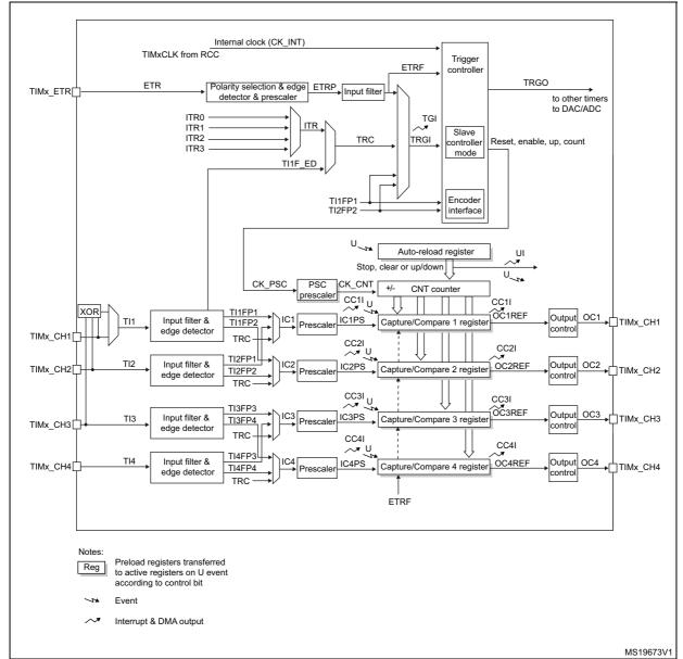
Figure 77. General-purpose timer block diagram
