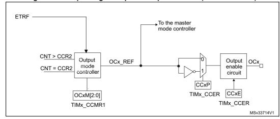
Figure 149. Output stage of capture/compare channel (channel 1 and 2)
