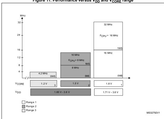
Figure 11. Performance versus V<sub>DD</sub> and V<sub>CORE</sub> range
