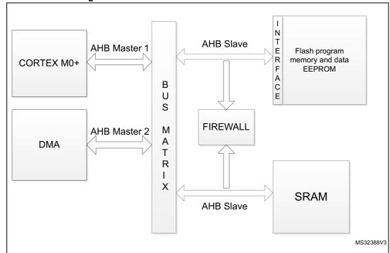
Figure 8. STM32L0x1 firewall connection schematics
