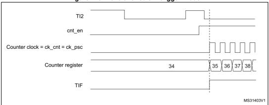
Figure 115. Control circuit in trigger mode
