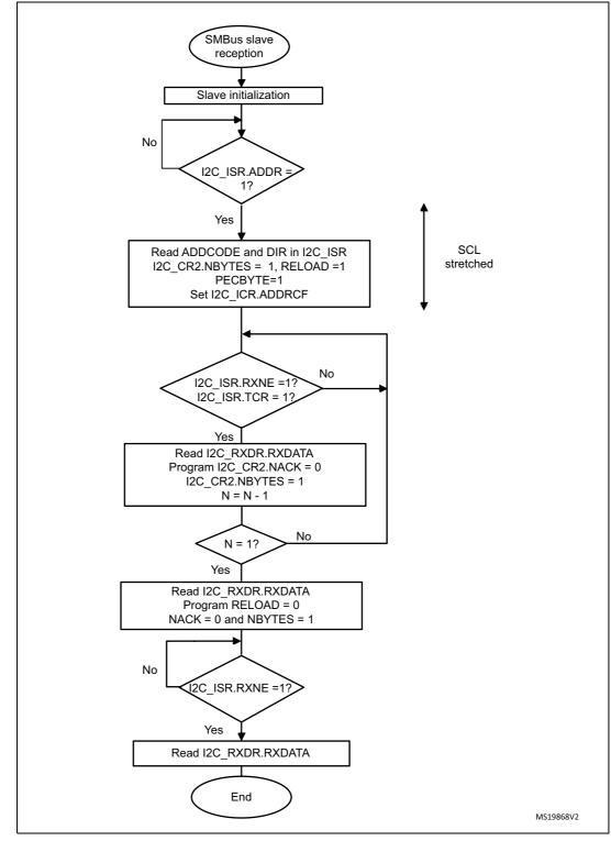
Figure 209. Transfer sequence flow for SMBus slave receiver N Bytes + PEC
