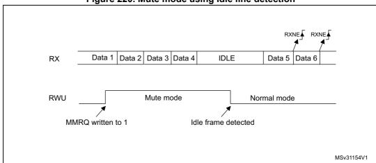
Figure 220. Mute mode using Idle line detection
