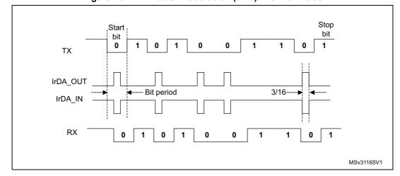
Figure 231. IrDA data modulation (3/16) -Normal Mode
