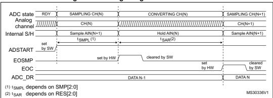
Figure 36. ADC conversion timings
