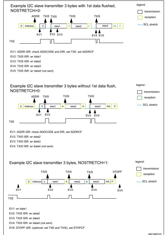
Figure 192. Transfer bus diagrams for I2C slave transmitter
