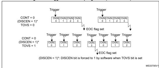
Figure 54. Triggered oversampling mode (TOVS bit = 1)
