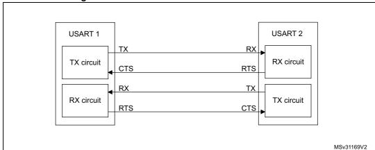
Figure 234. Hardware flow control between 2 USARTs
