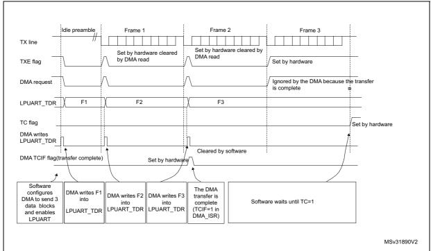
Figure 244. Transmission using DMA
