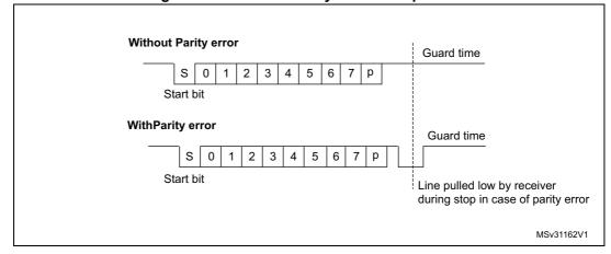
Figure 228. ISO 7816-3 asynchronous protocol
