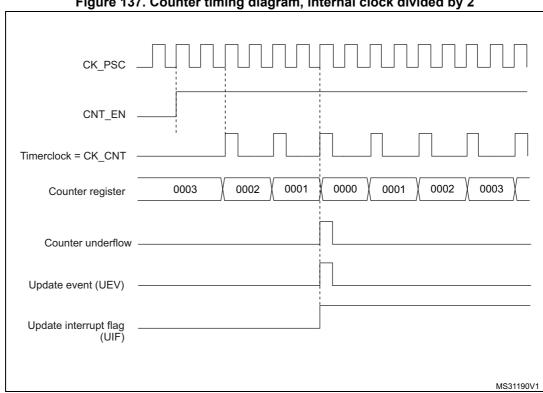
Figure 137. Counter timing diagram, internal clock divided by 2
