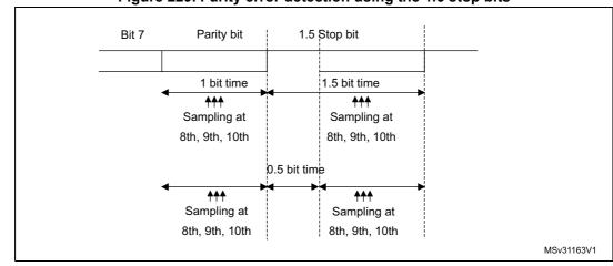
Figure 229. Parity error detection using the 1.5 stop bits
