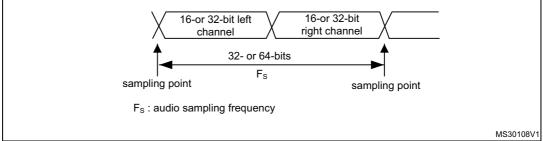
When the master mode is configured, a specific action needs to be taken to properly program the linear divider in order to communicate with the desired audio frequency.
