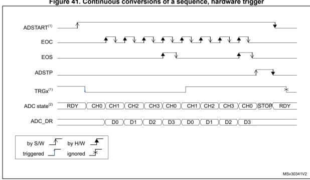
Figure 41. Continuous conversions of a sequence, hardware trigger
