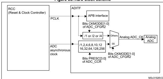
Figure 33. ADC clock scheme
