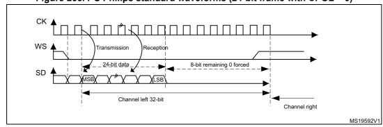
Figure 266. I<sup>2</sup>S Philips standard waveforms (24-bit frame with CPOL = 0)
