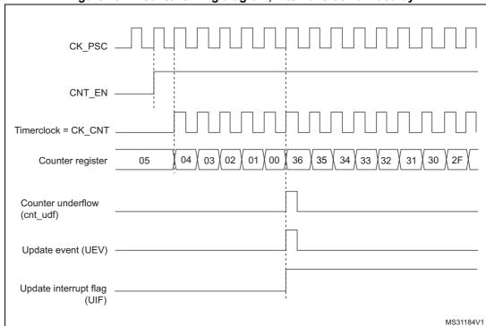
Figure 132. Counter timing diagram, internal clock divided by 1
