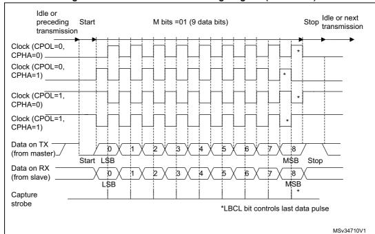
Figure 226. USART data clock timing diagram (M bits = 01)
