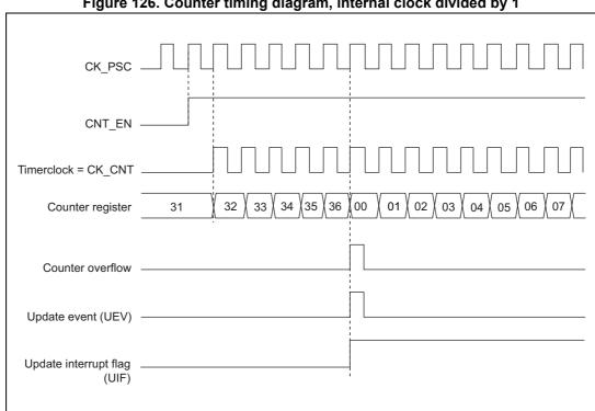
Figure 126. Counter timing diagram, internal clock divided by 1
