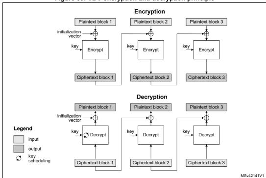
Figure 59. CBC encryption and decryption principle
