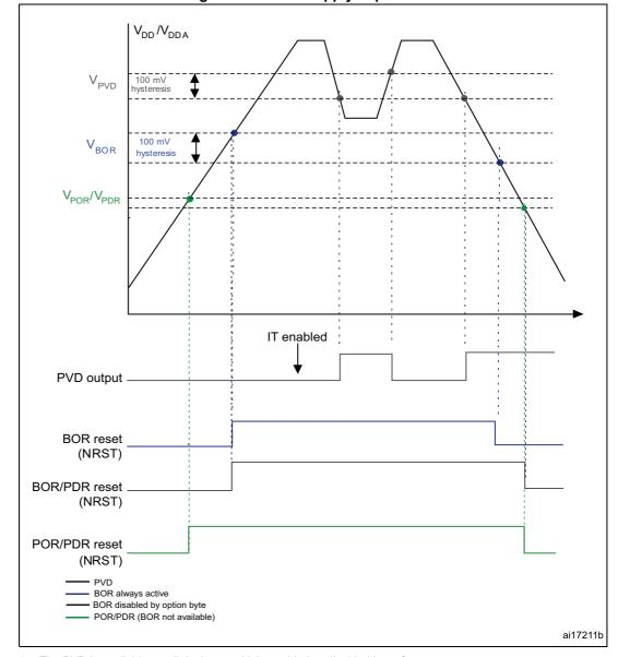
Figure 12. Power supply supervisors
