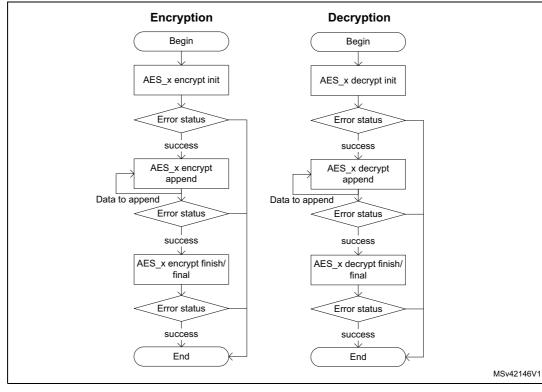
Figure 61. STM32 cryptolib AES flowchart example
