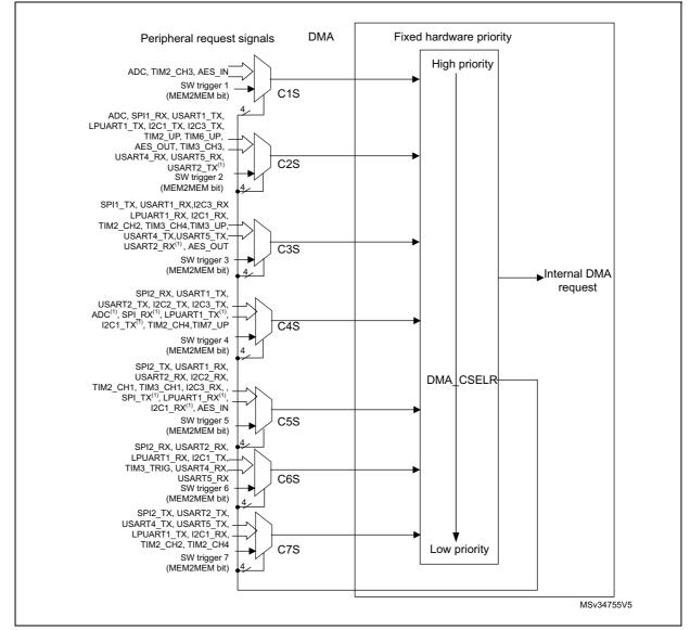
Figure 25. DMA request mapping
