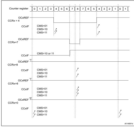
Figure 108. Center-aligned PWM waveforms (ARR=8)
