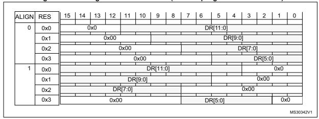
Figure 42. Data alignment and resolution (oversampling disabled: OVSE = 0)
