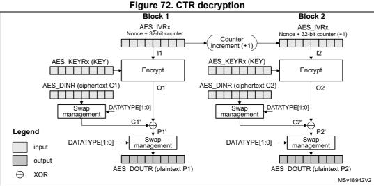
In CTR mode, the cryptographic core output (also called keystream) Ox is XOR-ed with relevant input block (Px' for encryption, Cx' for decryption), to produce the correct output block (Cx' for encryption, Px' for decryption). Initialization vectors in AES must be initialized as shown in Table 69.
