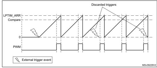
Figure 175. LPTIM output waveform, Continuous counting mode configuration
