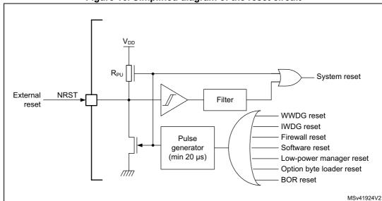
Figure 16. Simplified diagram of the reset circuit
