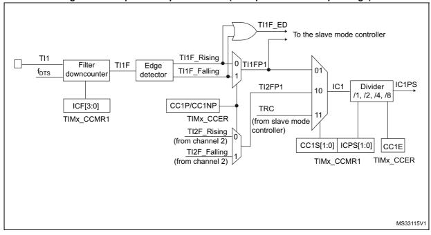
Figure 102. Capture/compare channel (example: channel 1 input stage)
