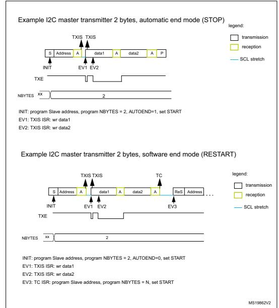
Figure 202. Transfer bus diagrams for I2C master transmitter
