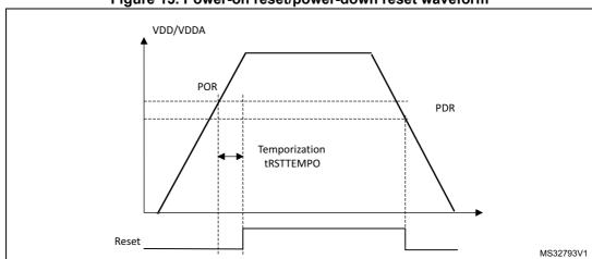
Figure 13. Power-on reset/power-down reset waveform
