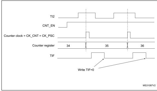
Figure 144. Control circuit in external clock mode 1
