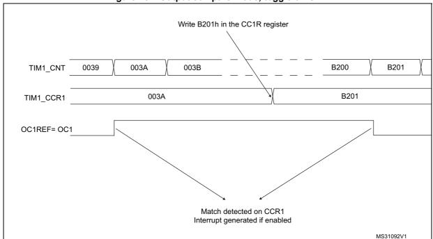
Figure 151. Output compare mode, toggle on OC1
