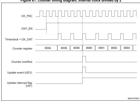
Figure 81. Counter timing diagram, internal clock divided by 2
