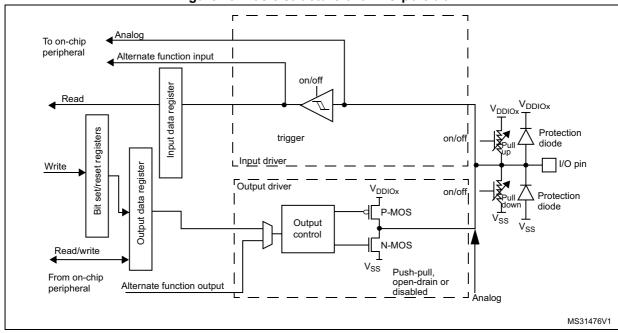
Figure 19. Basic structure of an I/O port bit
