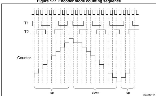
Figure 177. Encoder mode counting sequence
