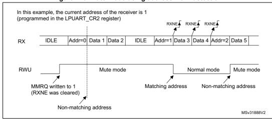
Figure 243. Mute mode using address mark detection
