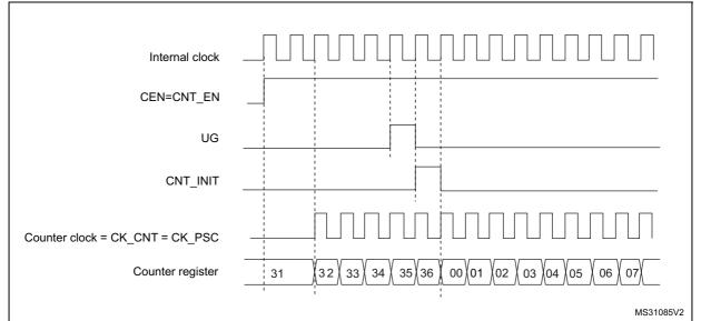
Figure 170. Control circuit in normal mode, internal clock divided by 1
