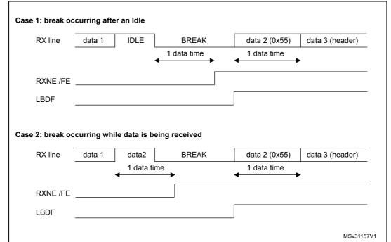
Figure 223. Break detection in LIN mode vs. Framing error detection
