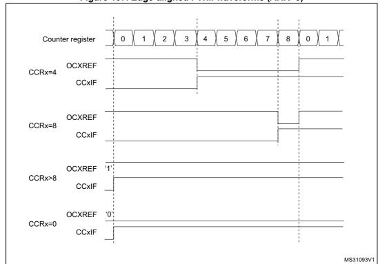
Figure 107. Edge-aligned PWM waveforms (ARR=8)
