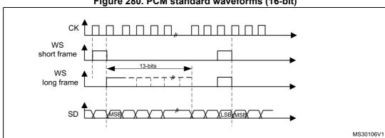
Figure 280. PCM standard waveforms (16-bit)
