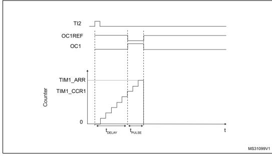
Figure 155. Example of one pulse mode
