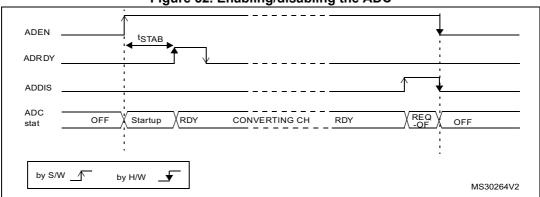
Figure 32. Enabling/disabling the ADC
