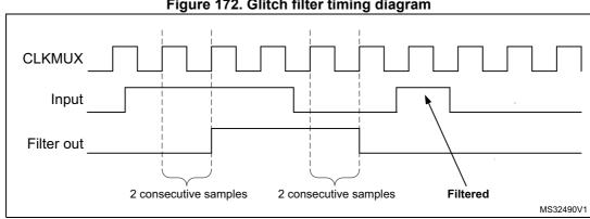
Figure 172. Glitch filter timing diagram
