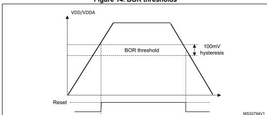
Figure 14. BOR thresholds
