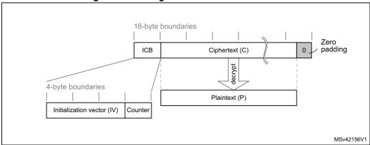
Figure 70. Message construction in CTR mode
