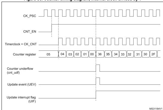
Figure 86. Counter timing diagram, internal clock divided by 1
