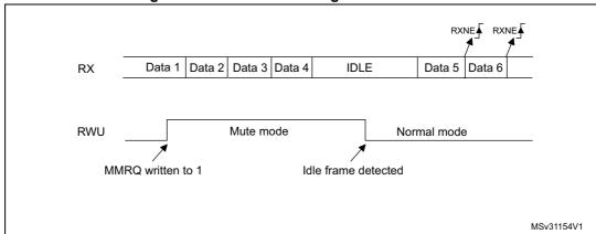
Figure 242. Mute mode using Idle line detection
