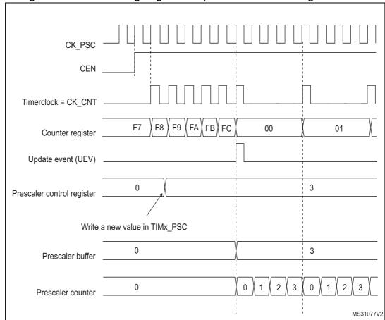
Figure 125. Counter timing diagram with prescaler division change from 1 to 4
