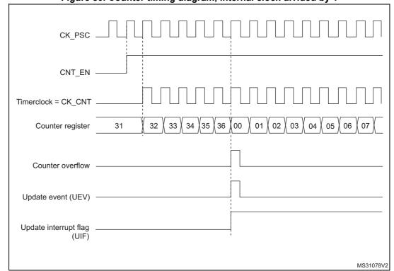
Figure 80. Counter timing diagram, internal clock divided by 1
