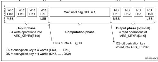
Figure 62. Encryption key derivation for ECB/CBC decryption (Mode 2)
