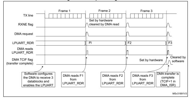
Figure 245. Reception using DMA
