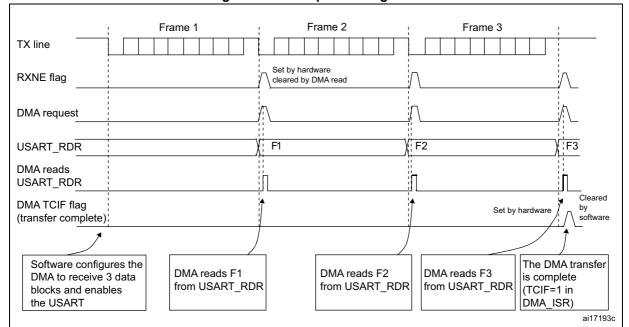
Figure 233. Reception using DMA
