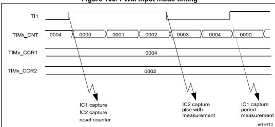
Figure 105. PWM input mode timing
