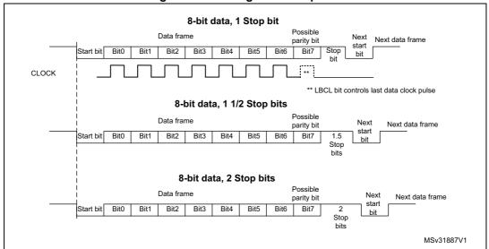
Figure 215. Configurable stop bits
