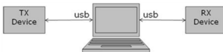
Figure 4. Connection setup 1: 1 PC with S2-LP-DK GUI
