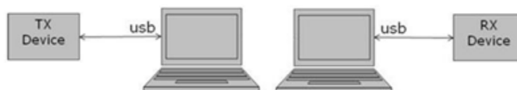
Figure 5. Connection setup 2: 2 PCs with S2-LP-DK GUI
