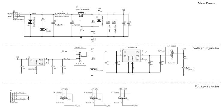
Figure 3: AEK-AUD-C1D9031 circuit schematic (3 of 6)
