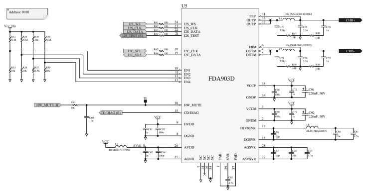
Figure 6: AEK-AUD-C1D9031 circuit schematic (6 of 6)
