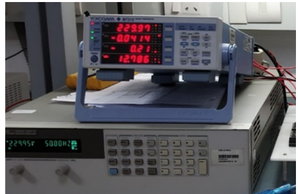
Figure 26. Standby power consumption: 0.21 W at nominal input voltage
