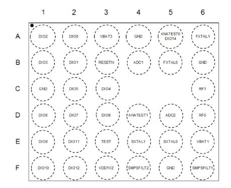
Figure 22. BlueNRG-1 ball out top view (WCSP34)
