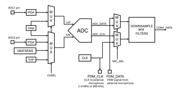
Several channels are available for the conversion, the CHSEL selects the channel according to Table 20. ADC channels.
