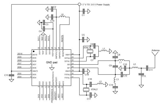
Figure 25. Application circuit: non-active DC-DC converter QFN32 package
