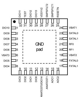
Figure 21. BlueNRG-1 pin-out top view (QFN32)
