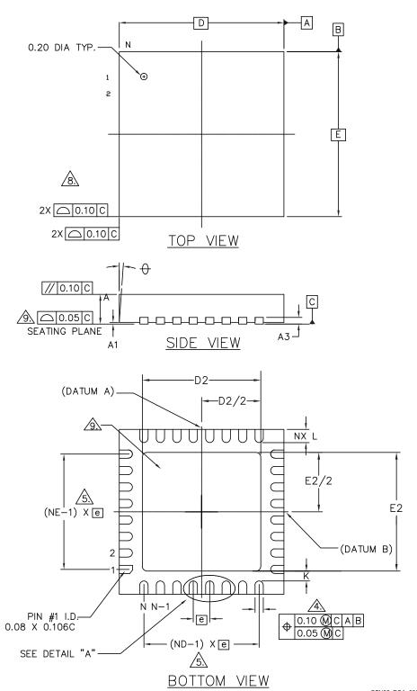
Figure 33. QFN32 (5 x 5 x 1 pitch 0.5 mm) package outline
