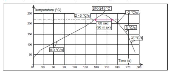
Figure 36. Flip Chip CSP (2.71 x 2.58 x 0.5 pitch 0.4 mm) package reflow profile recommendation
