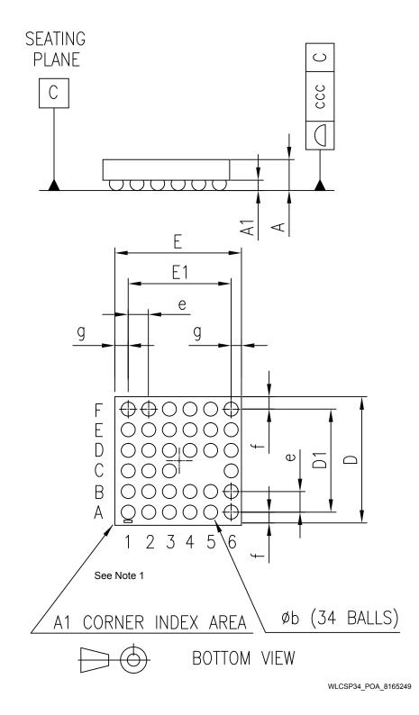
1. The corner of terminal A1 must be identified on the top surface by using a laser marking dot.
