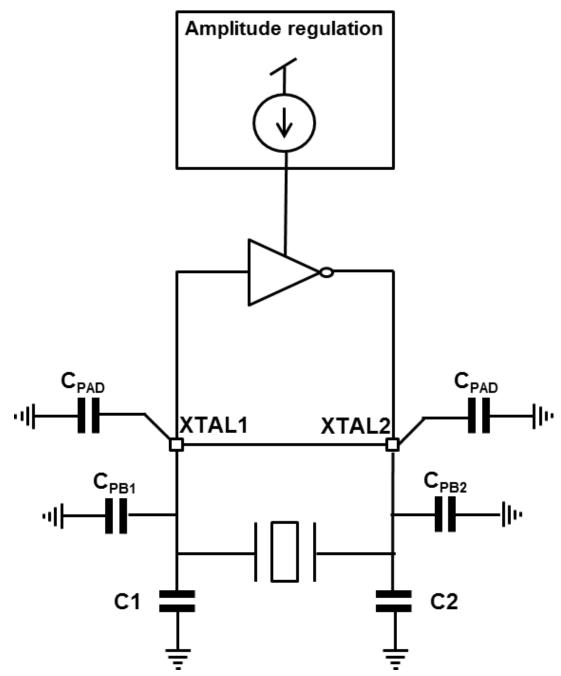
Figure 29. High speed oscillator block diagram
