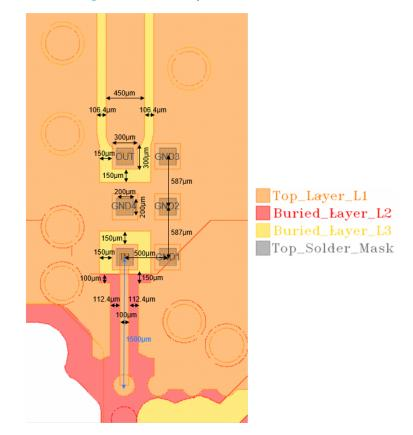
Transmission line between MLPF and antenna is dimensioned to 50 ohms characteristic impedance. Transmission line between STM32 and MLPF is dimensioned to 56 ohms characteristic impedance. Theses transmission line characteristics impedances have to be followed as close as possible. Moreover, lines physical dimensions will have to be tuned according to specific PCB stack up if different from the one presented in datasheet to keep expected characteristic impedance values.
