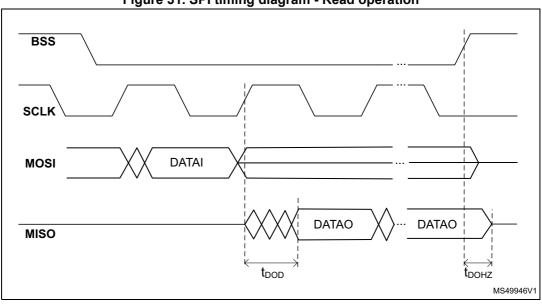
Figure 31. SPI timing diagram - Read operation
