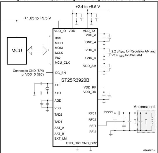
Figure 1. Minimum system configuration - Single sided antenna driving
