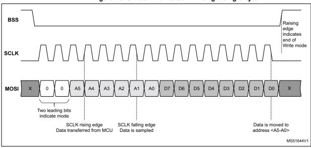
Figure 13. SPI communication: writing a single byte
