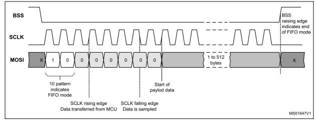
Figure 16. SPI communication: FIFO loading
