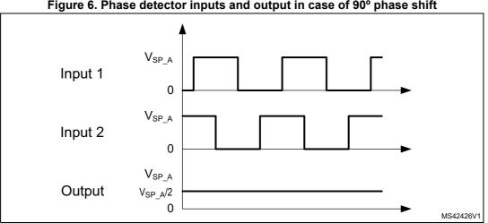
Figure 6. Phase detector inputs and output in case of 90° phase shift
