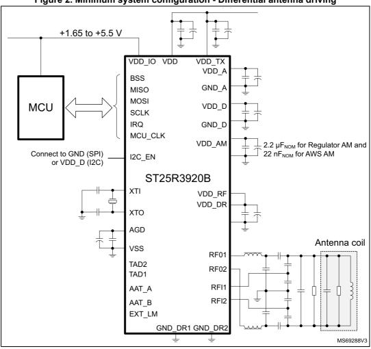
Figure 2. Minimum system configuration - Differential antenna driving
