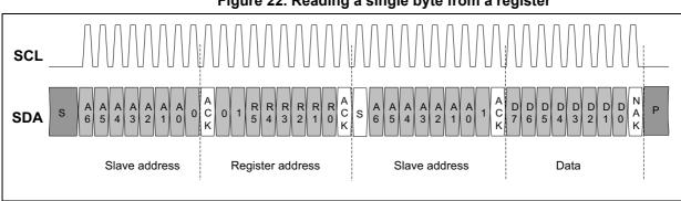
Figure 22. Reading a single byte from a register
