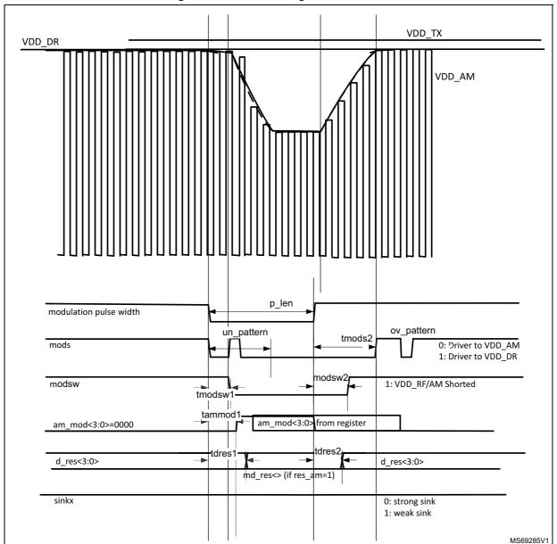
Figure 11. Bit and timing relation for ASK waveform
