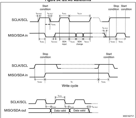
Figure 34. I2C AC waveforms
