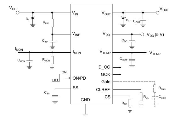
Figure 4. Typical application diagram (current limit fixed via R<sub>CL</sub>)
