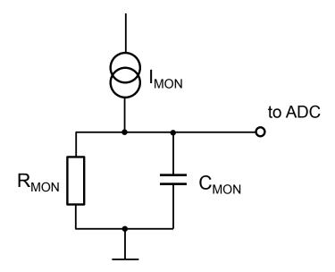
Figure 6. Current monitor simplified circuit
