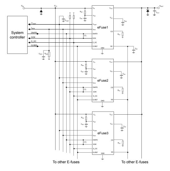
Figure 5. Typical application diagram (multiple e-fuses in parallel)
