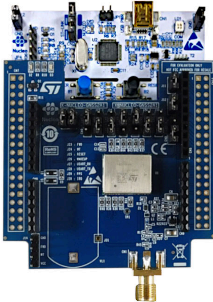
Figure 2. X-NUCLEO-GNSS2A1 expansion board connected to an STM32 Nucleo development board
