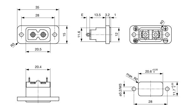
E: Solder terminals long: 7.3 mm (L=8.5 mm)
