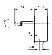
Cable diameter max. 4.0 mm
