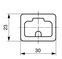
E: Solder terminals: 22.5 mm E: Quick connect terminals: 25.5 mm S: 1.5, 2.5, 3.0 mm
