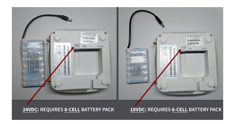
**NOTE:** The smaller, 6-cell battery pack will **NOT** power the 24V version of the MX.
