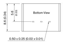
Dimensions in mm (inch) Tolerances:  $x.xx \pm 0.5 (\pm 0.02)$ Tolerances:  $x.xxx \pm 0.25 (\pm 0.01)$ Pin dimension tolerances: ±0.10 (±0.04)
